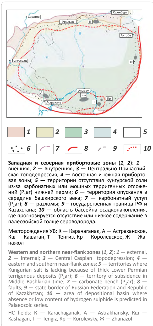
Fig. 7. Zoning of Palaeozoic sequence and prediction of accumulations with low content of hydrogen sulphide in them (prepared by Azhgaliev D.K. according to Obryadchikov O.S., 2018)
