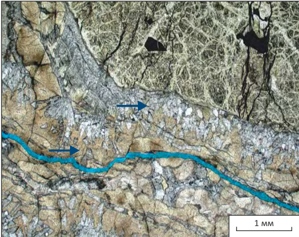
Fig. 8. Pores in magnesite aggregates (Gerasimovsky area, Gerasimovsky C well. Magnification 25, II nicols)
