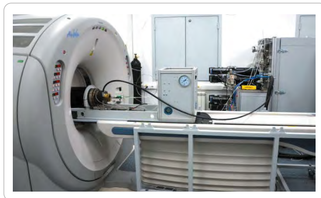
Fig. 3. Waterflood laboratory setup with CT-scanner
