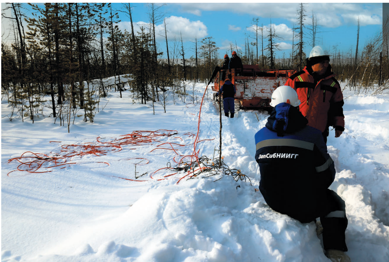
Fig. 7. Unreeling a receiver line during seismic data acquisition at the South Visimsky site
