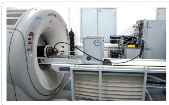
Fig. 3. Waterflood laboratory setup with CT-scanner
