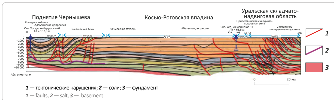
Fig. 2. Geological and geophysical model of structure of the Urals Foredeep northern segment (according to materials of Severgeofizika)
