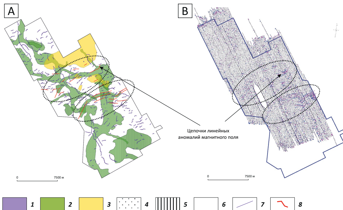
Fig. 9. Comparison of 3D seismic data interpretation in the near-surface and high-frequency component of magnetic field
