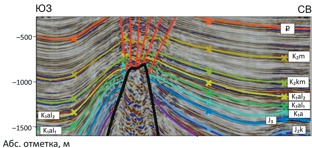
Fig. 8. Faults within the salt domes
